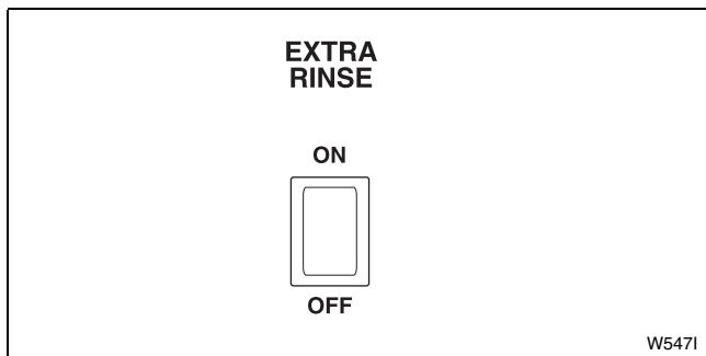
The EXTRA RINSE control is useful for detergent sensitive skin. By pressing the EXTRA RINSE to ON, the REGULAR, PERMANENT PRESS, and DELICATE cycles will each provide an additional rinse. If the extra rinse is desired, press the switch to ON. When the extra rinse is not wanted, OFF should be selected.
